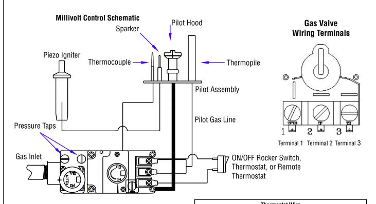
CAUTION: Label all wires prior to disconnection when servicing controls. Wiring errors can cause improper and dangerous operation. Verify proper operation after servicing.
